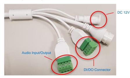
**NOTE:** If these connectors will not be used, make sure to wrap them with waterproof tape to avoid water or dust from entering the connectors.
