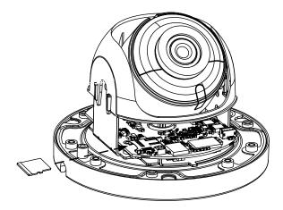
**NOTE**: In case there is a need to remove the card, make sure to access the camera Web Configurator to safely "unmount" the card first (see the camera Firmware User's Manual for more information). Once unmounted from the firmware, pull the card from the slot.
