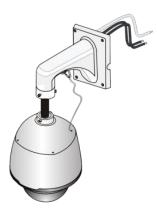
Attach the dome to the bracket adapter.
