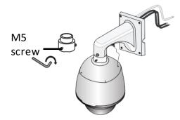
6. Connect the cables and attach the bracket to the wall with flat pads, washers and nuts.
