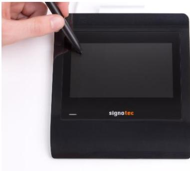
Touch the display with the pen at the **top left-hand corner**. While holding the pen, reconnect the pad to the power supply. After booting successfully, the LED switches from red to orange.
