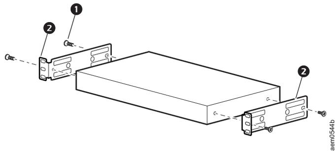
3. Secure the appliance to the rack, using cage nuts and screws (not provided).
