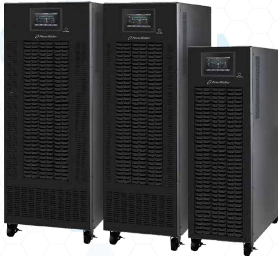
The PowerWalker VFI CPG 3/3 PF1 series is a professional commercial solution built in double conversion technology with power factor 1.0. Equipped with three-level inverter topology, it results in a high efficiency, reaching 95.5% in Line Mode and even 98.5% in ECO Mode. The series ensures low harmonic distortions and precise voltage regulation (1%). All phases have Active Power Factor Correction.
