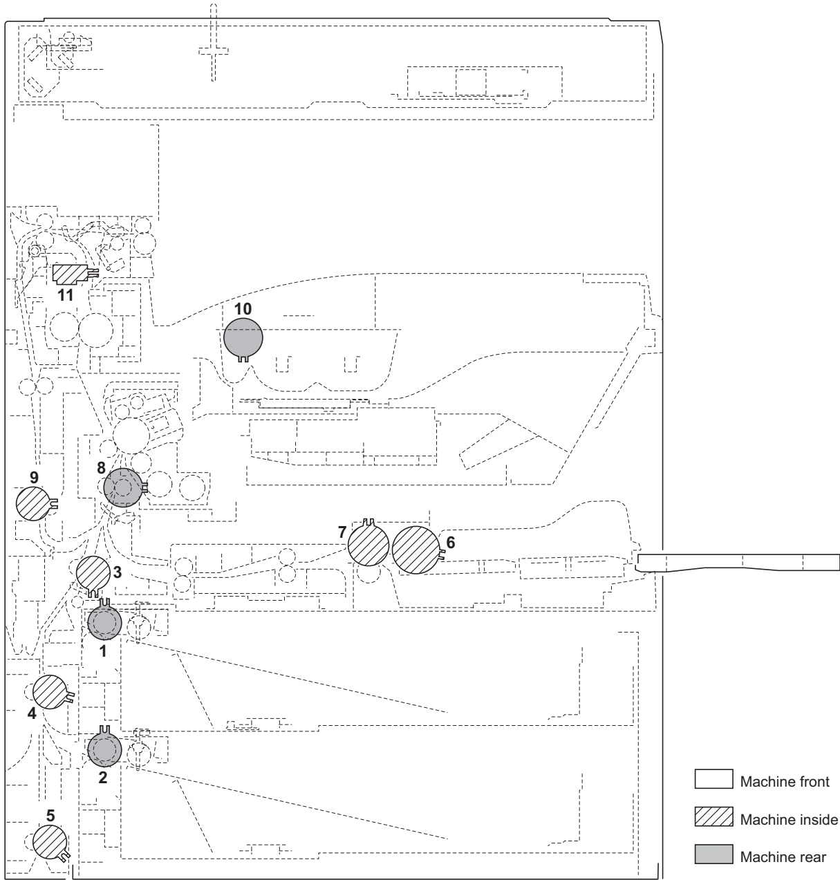
Figure 2-2-4 Clutches and solenoids
