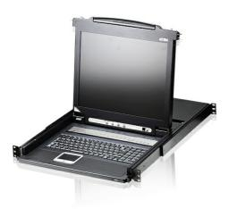
The CL1016 LCD KVM Switch series are control units that allow access to multiple computers from a single keyboard, video, and mouse (KVM), console. A single CL1016 can control up to 16 computers. As many as 15 additional KVM switches can be daisy-chained to the CL1008, so that up to 256 computers can all be controlled from a single KVM console.
