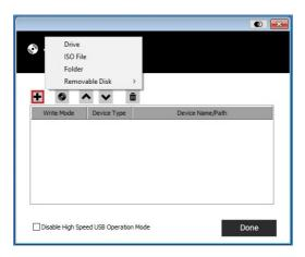
If the device only supports full speed USB, please check the Disable High Speed USB Operation Mode box.
