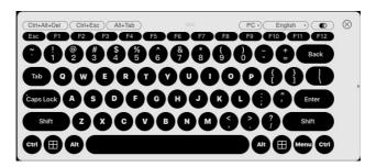
One of the advantages of the on-screen keyboard is that if the keyboard languages of the target computer and laptop's are not the same, then, there is no need to change settings of either system. Simply bring up the on-screen keyboard, selected the preferred language, and use the on-screen keyboard to type with.
