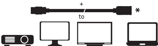
\*this is an extension cable intended to extend the existing cable length of your setup
