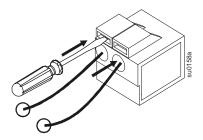
Both Class 2 and SELV circuits must be isolated from all primary circuitry. Do not connect any circuit to the EPO terminal block unless it can be confirmed that the circuit is Class 2 or SELV. If circuit standard cannot be confirmed, use a contact closure switch.
