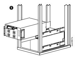
Secure the UPS and the XLBP(s) in the rack using the cage nuts and ornamental screws included in the package.
