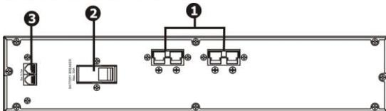
1. DC connector : connects to either UPS or 2<sup>nd</sup> battery box
