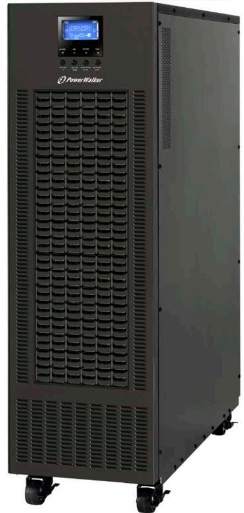
The PowerWalker VFI CPG 3/3 series is a professional commercial solution built in double conversion technology with a high power factor of 0.9. Equipped with three-level inverter topology, it results in high efficiency reaching 95% in Line Mode and even 98% in ECO Mode. The series ensures low harmonic distortions and precise voltage regulation (1%). All phases have Active Power Factor Correction.
